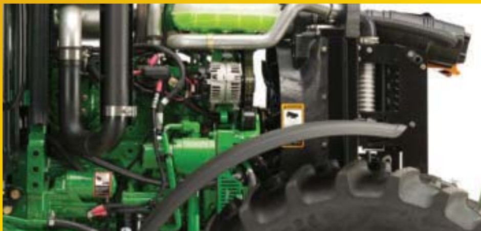
High-pressure common rail fuel (HPCR) injection system is standard on the 6115D, 6130D and 6140D.
